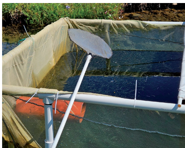
Figure 3b. A fry trap set up to record the migration of young salmon on the Gatchan River (photo by A.I. Barausov)
